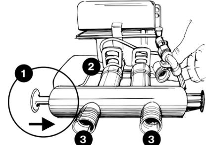
**RACCORDEMENT DE LA VANNE BYPASS**
