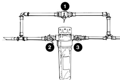
**RACCORDEMENT INSTALLATION CONFORME**
